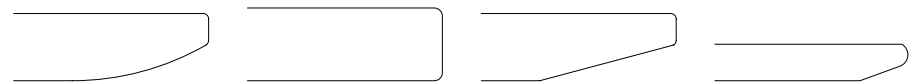
Solid wood lipping, rounded on the bottom, straight plastic lipping, chamfered wood lipping or chamfered HPL solid-core lipping
